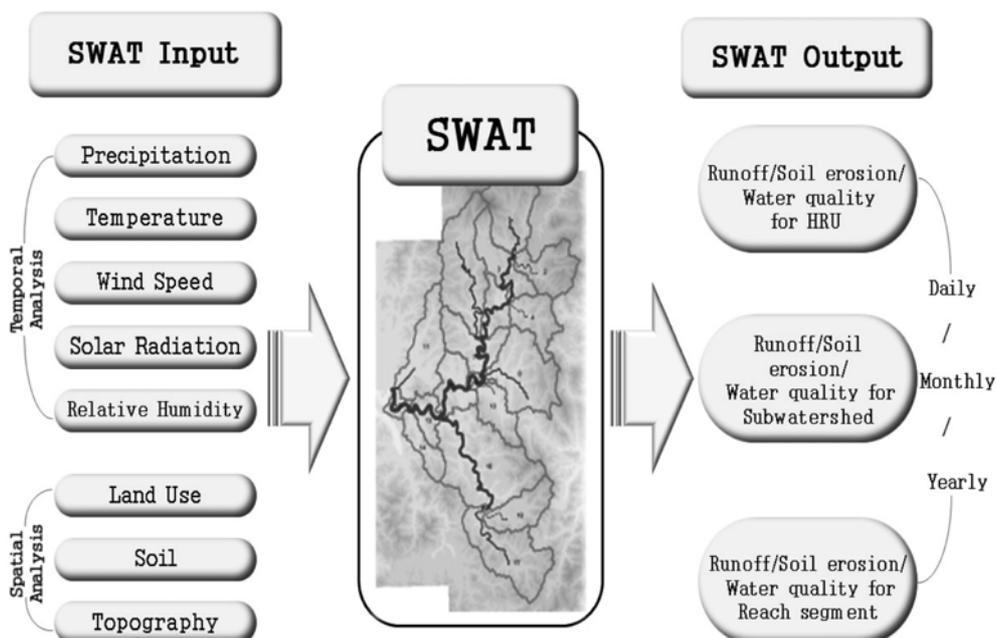
**Fig. 2.** Input and output data of SWAT.
