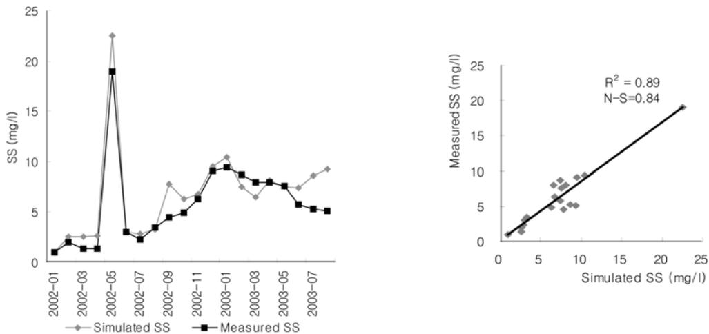
Fig. 9. Comparison of SWAT Estimated SS vs. Measured SS (2002. 01. ~ 2003. 08.).
