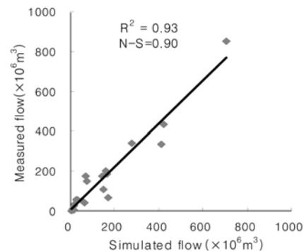
Fig. 7. Calibration of SWAT Hydrologic Component (2002. 01. ~ 2003. 12.).
