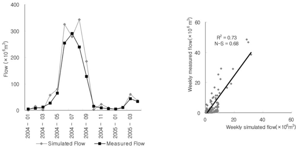
Fig. 8. Validation of SWAT Hydrologic Component (2004. 01. ~ 2005. 04.).
