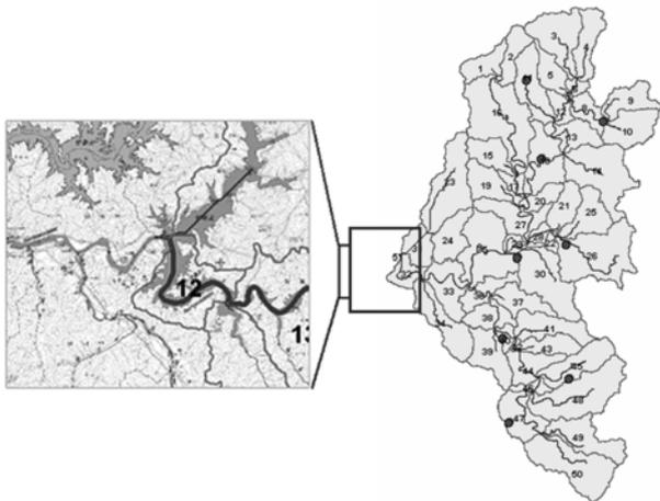
Fig. 6. Subwatershed delineation at Imha-dam watershed for SWAT run.
